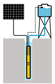
control pump start and stop, connecting a float switch, for example. All the protections against overload, surges and dry running are integrated into the on-board inverter.
