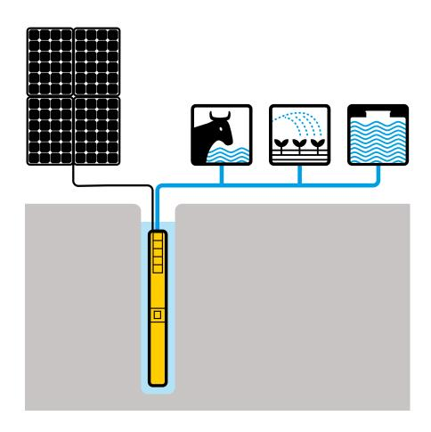
4HS MultiPower pump can be installed with CM MultiPower control module or without it, thus becoming a "plug and pump" system.
